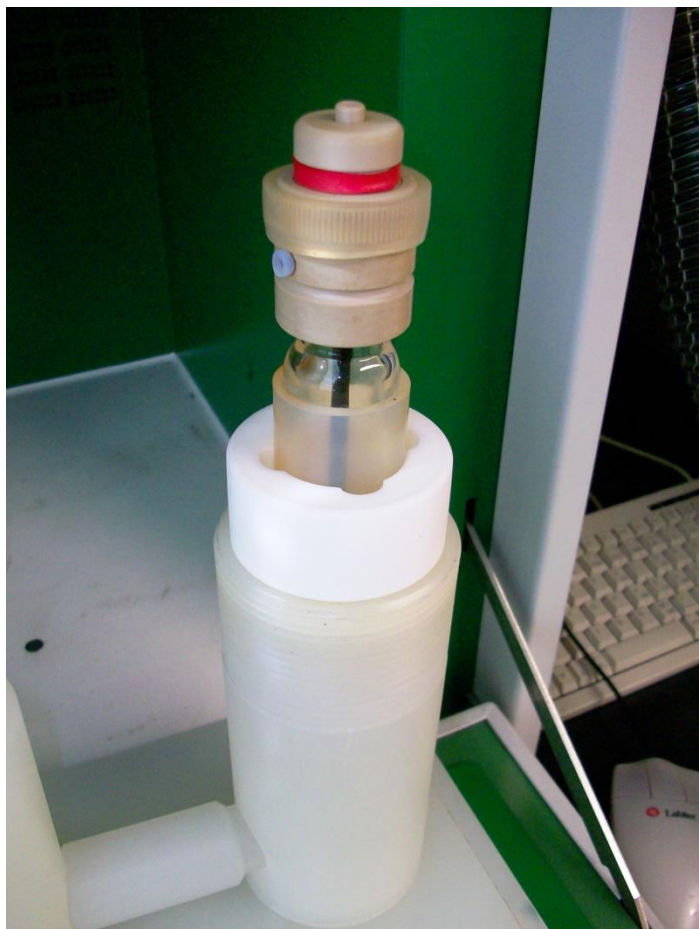
Place reactor tube in the teflon holder.
